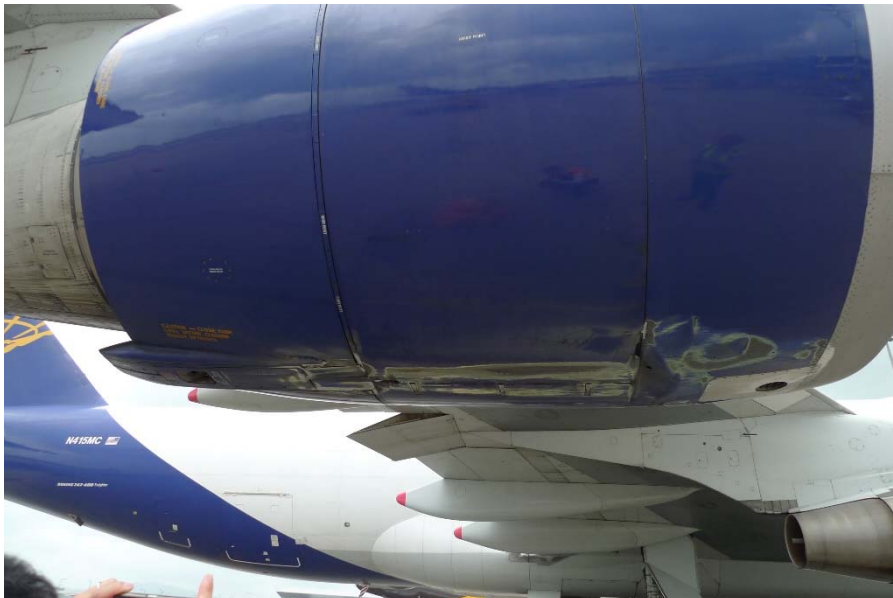
Photo 2: Damage at the Underside of No.4 Engine
