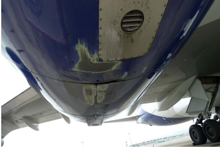
Photo 1: Damage at the Underside of No.3 Engine
